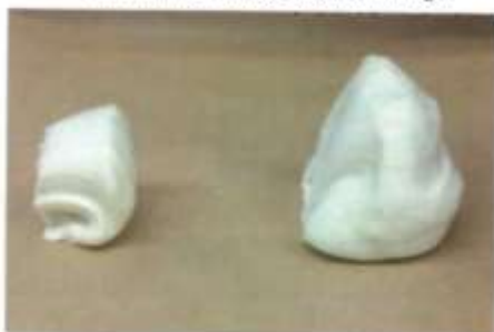
Fig. 3: SPF samples from flow testing. The sample on the left represents a low flowing sample versus a high flowing sample on the right
