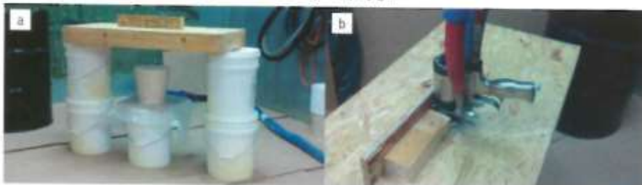
Fig. 4: a) spray table constructed for holding the Graco Fusion AP spray gun and the DFM-170 bucket; b) spray table with mounting bracket for holding the spray gun
