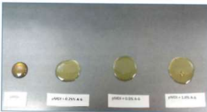
Fig. 9: 50 µl droplets of pMDI with and without A-6 surfactant. The surface area covered is significantly greater when A-6 is added to the pMDI versus standard pMDI.
