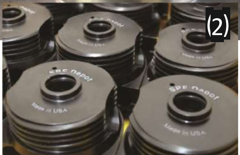
Video: laser etching is the final stage before SPF Depot's machined front ends (1) are finished (2); Below: Cutaways of a spray gun handle, a side seal, and mixing chambers
