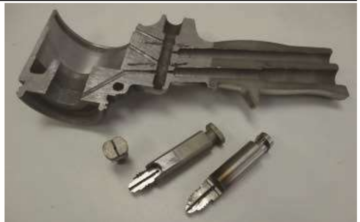
Video: laser etching is the final stage before SPF Depot's machined front ends (1) are finished (2); Below: Cutaways of a spray gun handle, a side seal, and mixing chambers
