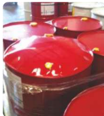
Figure 18 : B-side with water contamination
